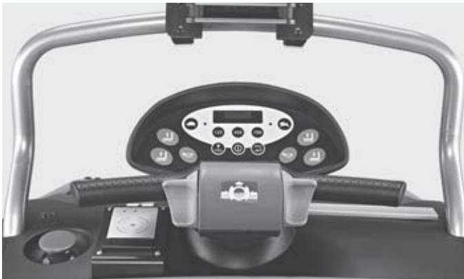
Everything within reach at all times: thanks to the STILL COCKPIT, both left and right-handed users can intuitively operate all of the truck's functions using ergonomic control elements 3
